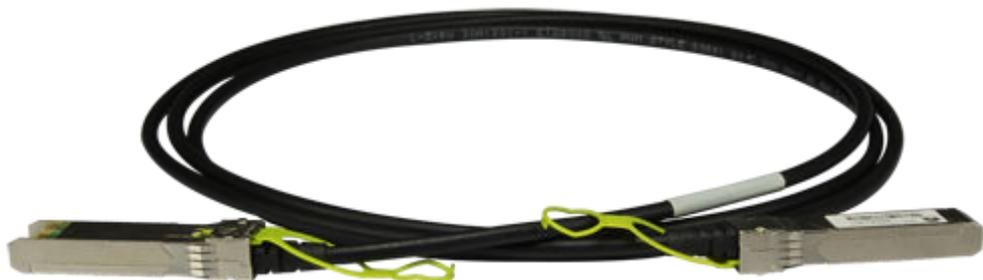
DACs are classified into active cables and passive cables. Active DACs have built-in amplifiers and equalizers to improve signal quality, but are expensive. In most cases, if the transmission distance is less than 5 m, passive DACs can be used. If the transmission distance is longer than 5 m, active DACs can be used.
