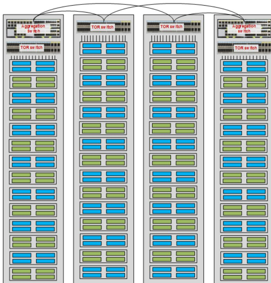
In the TOR architecture, each cabinet can be considered as an independent management entity. Servers and switches can be upgraded by cabinet. During upgrades, the traffic forwarding of other cabinets is not affected, and the impact on services is minimized.
